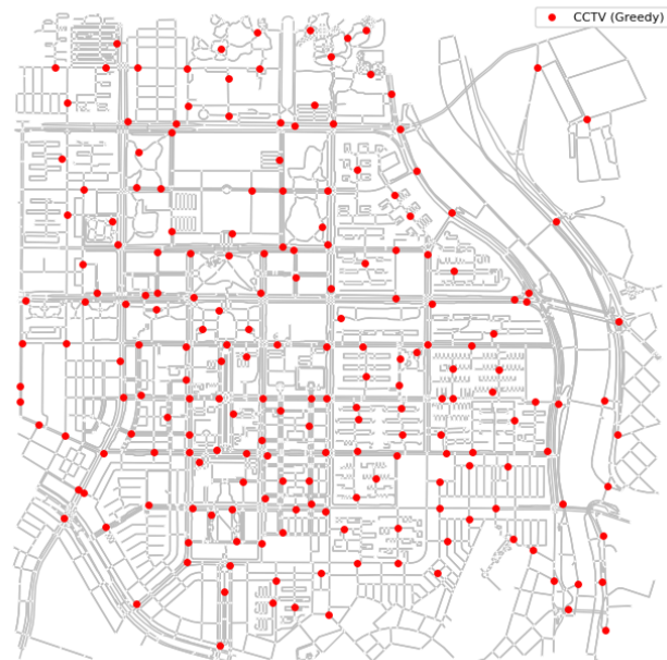
Figure 2. CCTV placement by Greedy algorithm
